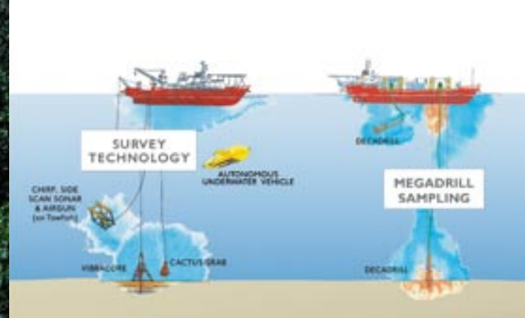
▲ The undersea prospecting will involve sampling seabed material by both core drilling and 'grab' techniques, with the material replaced after analysis on the research vessel.
