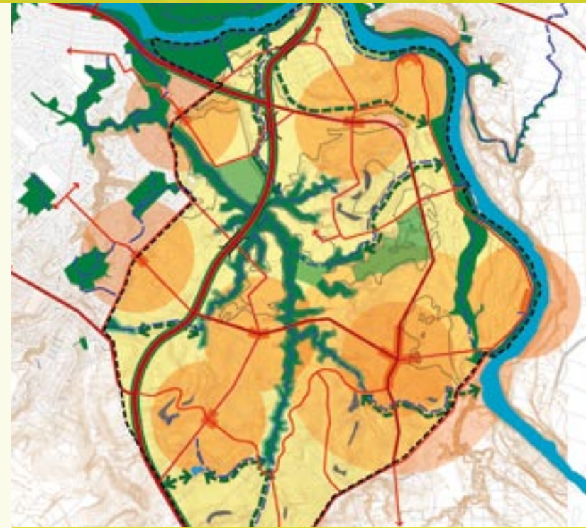
▲ The recommended option: a major arterial route provides a direct link to the city centre while a series of commercial centres – all within walking distance of green space – are linked by a secondary road network.
