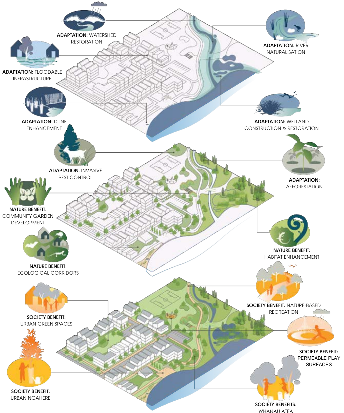
Figure 18: Common Nature-based Solutions and their associated co-benefits for nature and society across an urban blue-green network. Source: Boffa Miskell Ltd.
